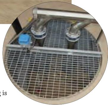
The OMEC system supplied by New Stone Age to Cumbrian Stone that can deliver 1,200 L/min of water, with back-up pumps throughout to ensure production continues if a pump fails.
